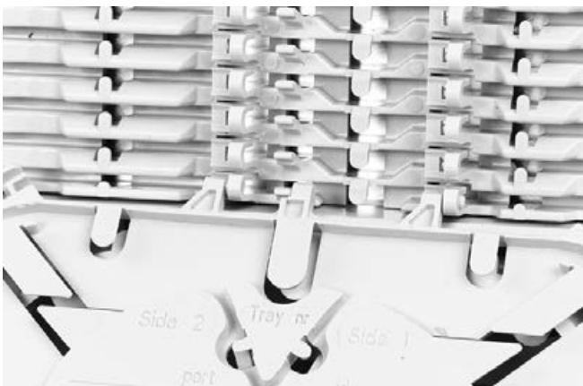
4.3 Place a tray in the wraparound groove plate; do this by pushing the lip on the groove plate (lowest possible position) slightly down with the tray and move the tray lateral into the hinge-cavities of the groove plate. To snap the High Capacity Single Element tray (HCSE) in the W/a single fiber groove plate leave always one hinge facility open between Fasblock or previous tray and the HCSE-tray.
